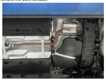
**Step 3.** Begin installation of your new MAGNAFLOW system by attaching the Inlet Muffler Assembly to the catalytic converter outlet using the OEM band clamp. Engage the welded hangers to the rubber insulators. Keep all fasteners and clamps loose until final adjustment.
