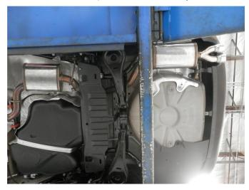
**Step 4.** Next use the supplied 2.25" clamp to loosely attach the Tailpipe Assembly to the Inlet Muffler Assembly. Finish by attaching the hangers into the rubber insulators.
